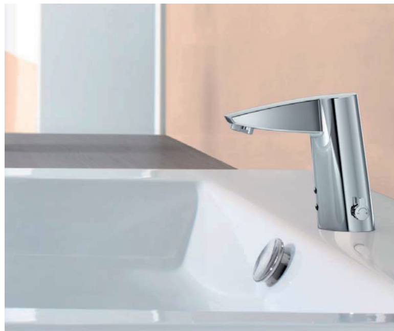
HANSALANO electronic washbasin mixer, DN 15 battery operated 6491 2210 chrome sensory electronic operation (infrared), without pop-up waste, flexible connection hoses, projection: 115 mm
